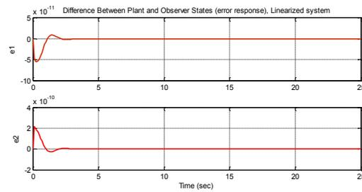
Figure 4: Responses of state errors e(t) when there is no fault in the system.
