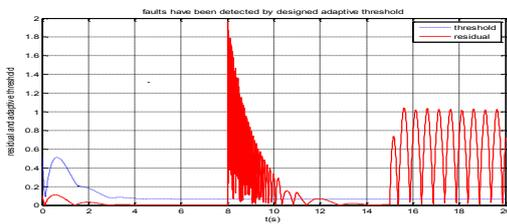
Fig 2: Adaptive threshold design when faults have been detected.
