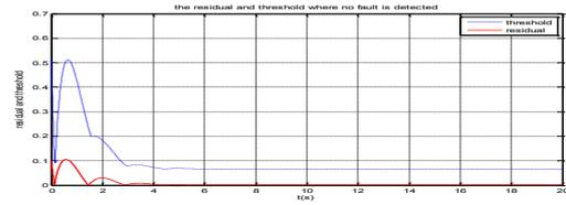
Fig 3: Adaptive threshold design when there is no fault to detect.
